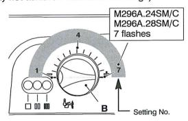
To change the setting, turn the hot water dial (B) to maximum setting 7
