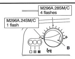
For a **24KW** turn the hot water dial **(B)** to **12 a clock** position and then **turn back** to **minimum** (the lockout lamp **(E)** will start to flash **twice per second**).
