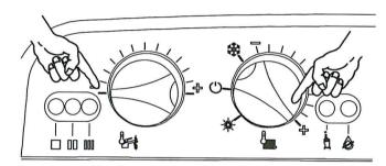
PRESS AND HOLD RESET/ LOCKOUT BUTTON FOR 10 SECONDS UNTIL LOCKOUT LIGHT STARTS TO FLASH
