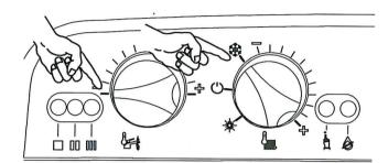
PRESS AND HOLD RESET BUTTON FOR 10 SECONDS UNTIL LOCKOUT LIGHT STARTS TO FLASH
